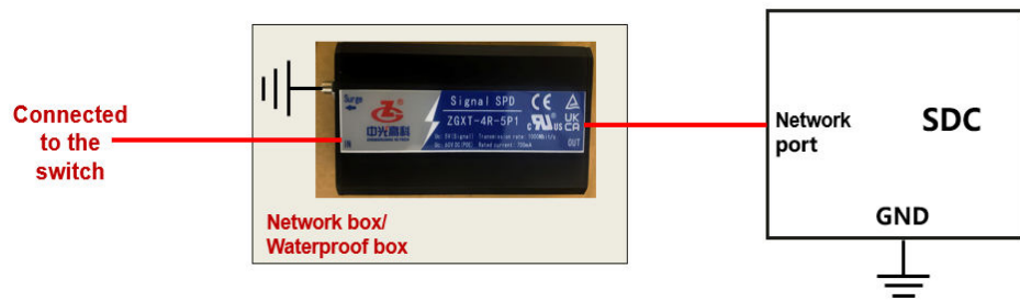
Figure A-4 Installation specifications for the network port surge protector
